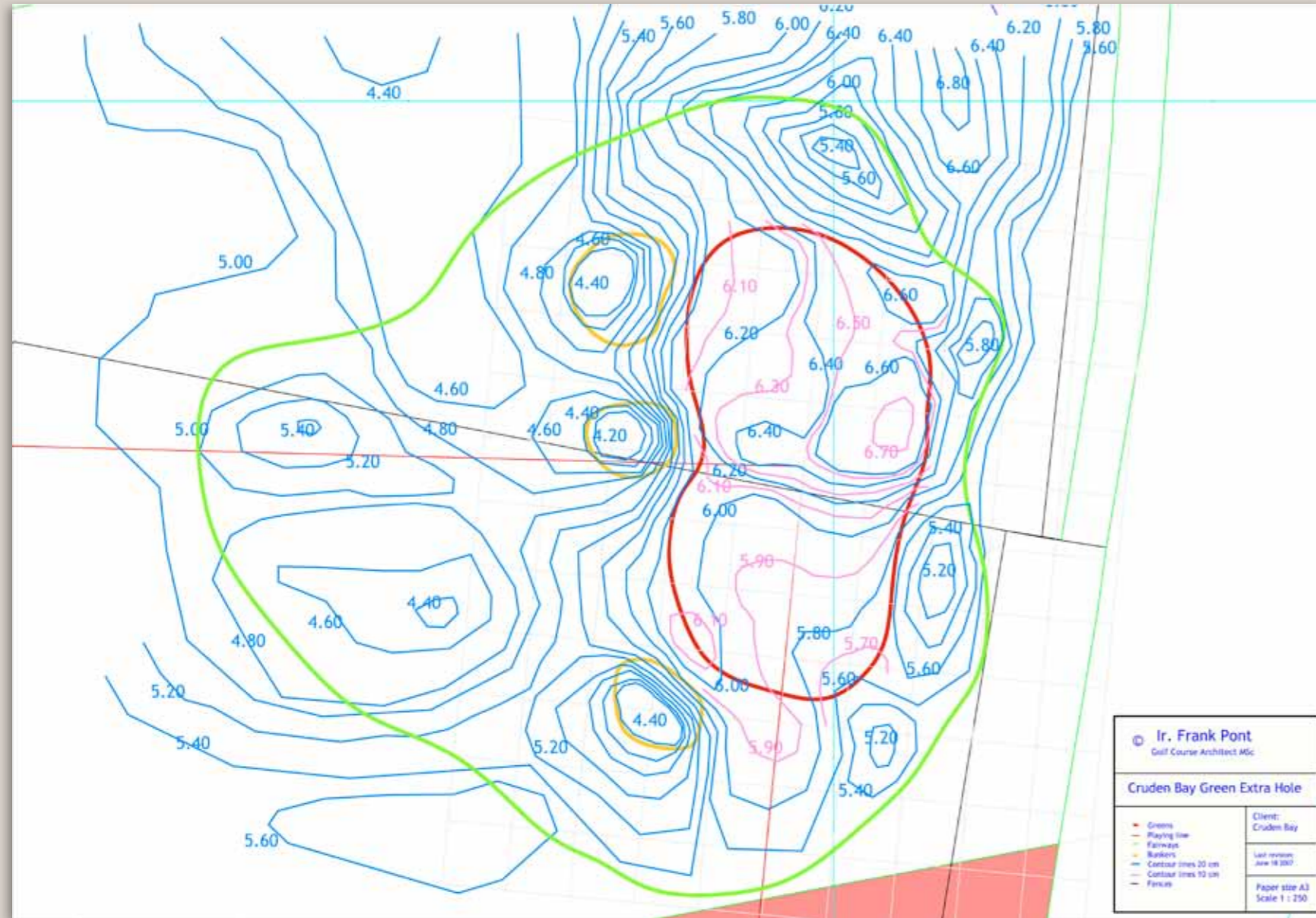
A detailed contour map of Sancraggs: note how the left portion of the green clearly slopes towards the player, while the right side of the green slopes away. Photograph by Frank Pont.
